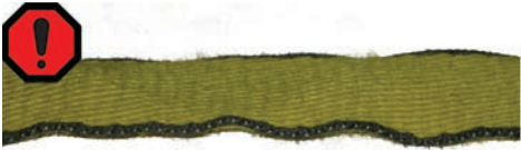
Heavy wear throughout, wavy edges Lanyard edges wavy, fabric breaking down, becoming dry and/or fading. Heavy use Dragging over an edge.
