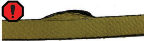
Edge wear and fraying Being dragged over an edge, improper mounting or accidental damage.
