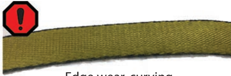
Edge wear, curving Dragging over an edge or improper mounting.
